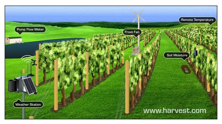
The Harvest system is an internet based online (IoT) solution covering a range of applications. In most situations, our systems are totally standalone utilising solar power and the cellular network to send data to the Harvest servers. Wireless UHF radio "remotes" can also be used to collect data from around the property. The information can be viewed using any computer or smartphone.
