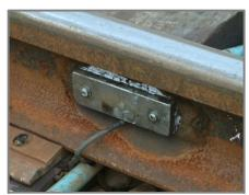
Figure 1 - Track Temperature Sensor
