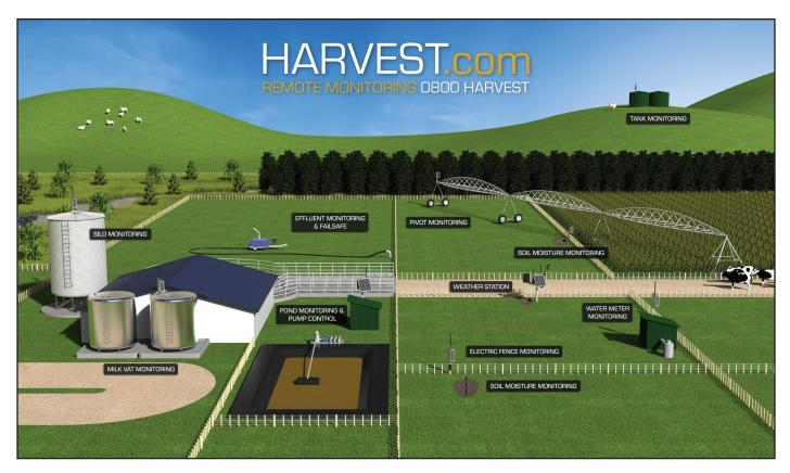
The Harvest system is an internet based (IoT) remote monitoring solution covering a range of applications. In most situations, our systems are totally standalone utilising solar power and the cellular network to send data to the Harvest servers. Wireless UHF radio "remotes" can also be used to collect data from around the property. The information can be viewed using any computer or smartphone.
