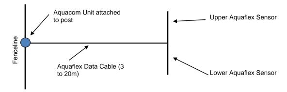
Figure 1.0 Aquaflex Installation Diagram
